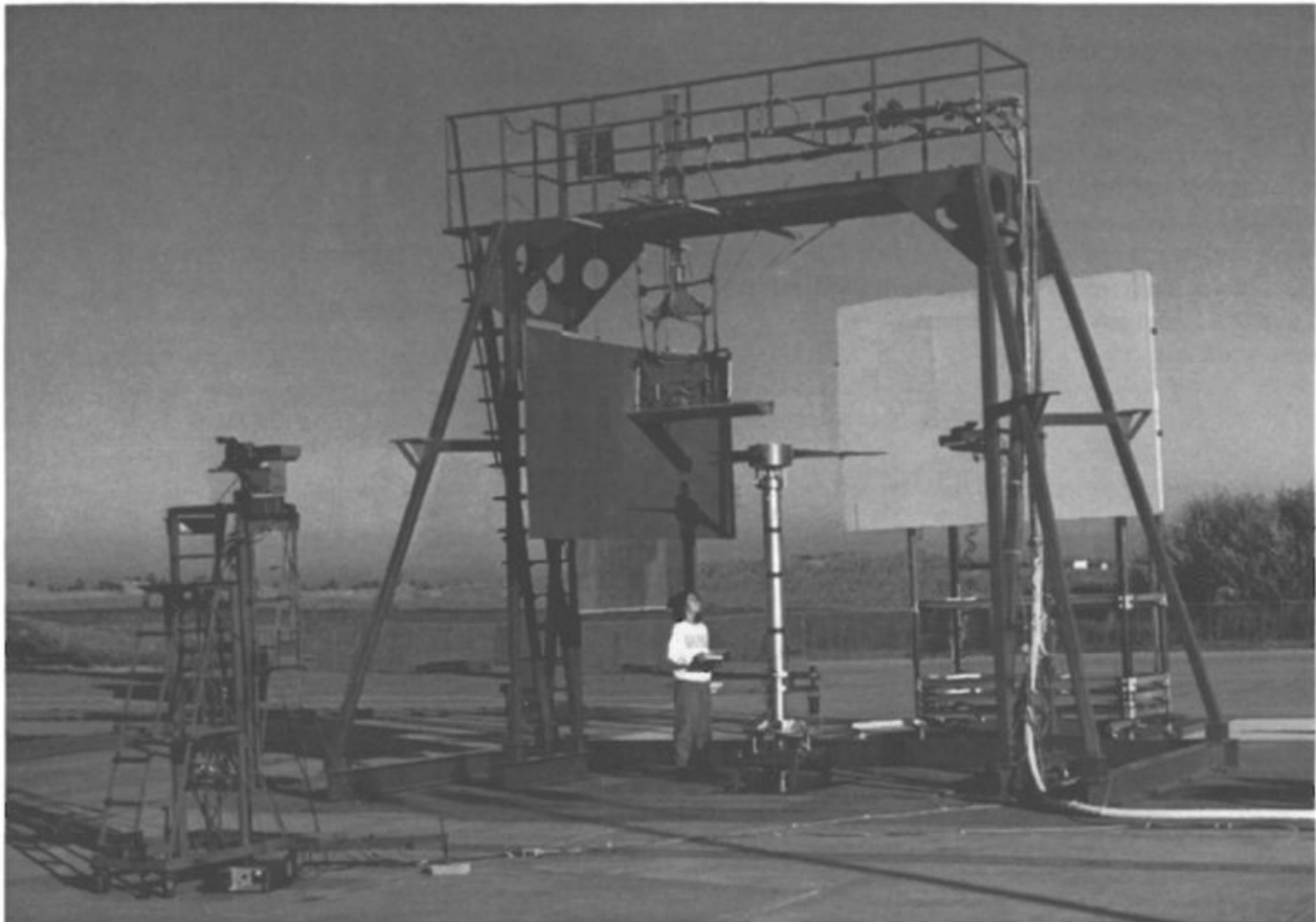
Figure 1a. Shadowgraph test installation at the Outdoor Aerodynamic Research Facility
